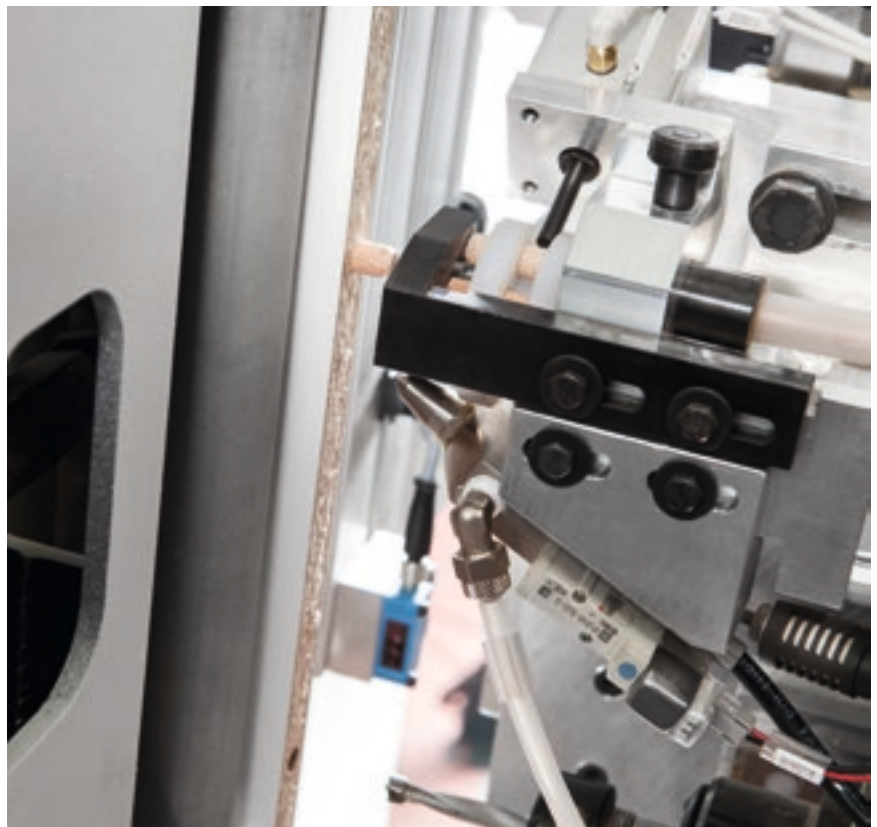
Unit for managing the drilling operation and the insertion of glue and dowels.
